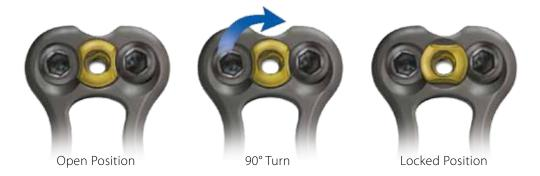
The locking mechanism is engaged with the same driver as the bone screws. A 90° clockwise turn securely locks both screws.
