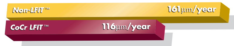
Figure 3 LFIT™ heads demonstrated a 28% reduction in linear wear over CoCr heads
