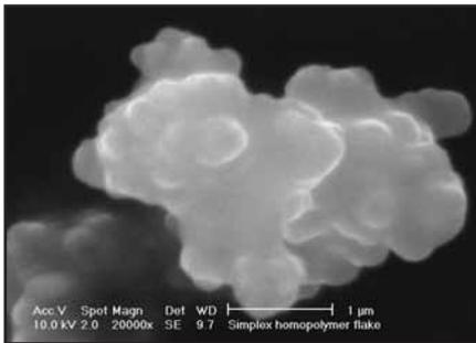
Methylmethacrylate is processed to form the PMMA 'flake' designed to increase wettability and improve handling characteristics.<sup>1</sup>
