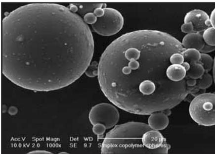
Styrene and methylmethacrylate are combined via a proprietary manufacturing process to form beads of varying size.
